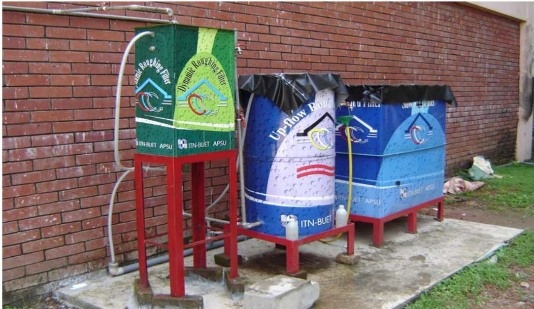
**Plate 2.1: Front View of the Laboratory Multistage Filtration Units**
