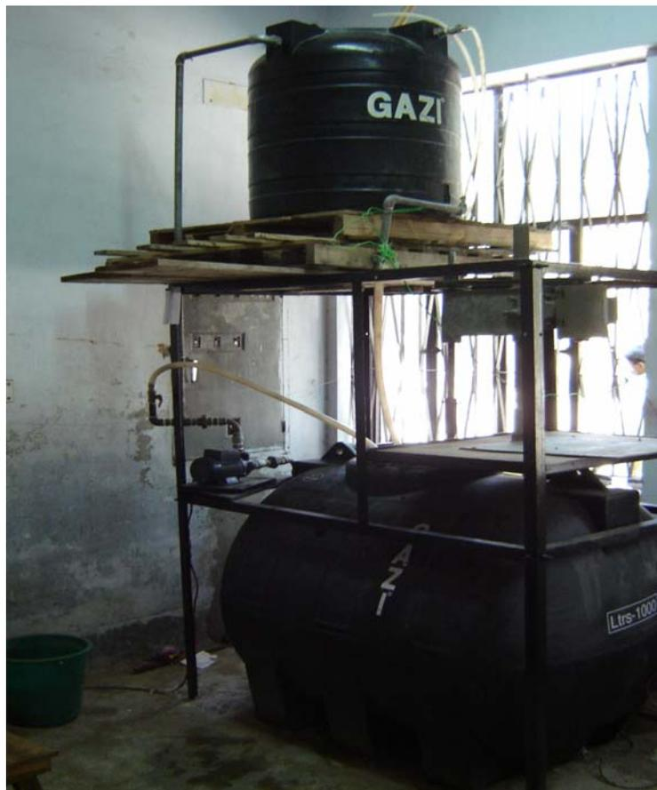
**Plate-2.2: Laboratory Raw water Feeding Arrangement to MSFs**
